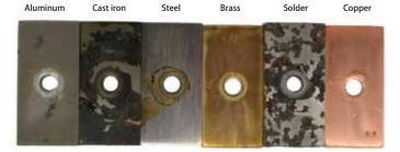
There are lots of corrosion on many of the test pieces which can cause overheating due to corrosion clogging, leakage etc of the radiator.
